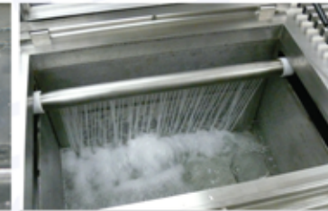
2/ rinse with automated horizontal travel
